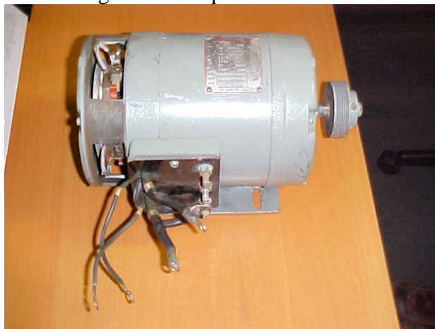
Figure 1: Compound DC Motor
